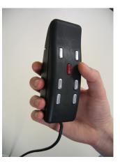
Figure 10: The modified Twiddler keypad used for input.
