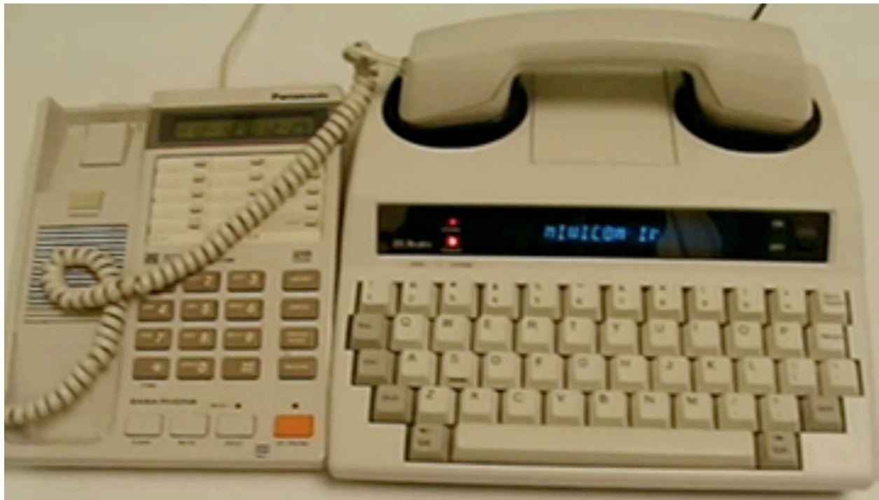
Figure 1: An Ultratec Minicom iV acoustically coupled TTY and a standard office phone used for initial testing.
